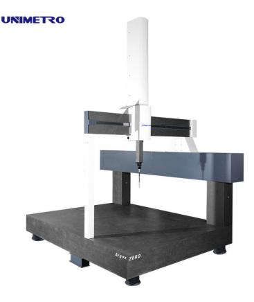
The krypton series CMM supports a variety of measurement methods, including triggered digital probe measurement, continuous contact analog probe scanning and laser probe scanning. All of these probe options are completely interchangeable, which helps to measure geometric parts and free shape parts.
